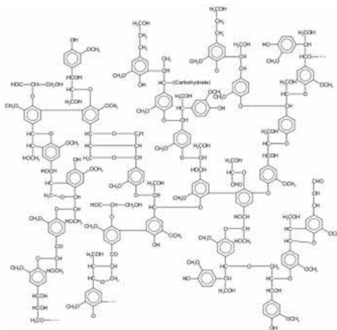
**Figure 1.** Representative section of the lignin macromolecule
