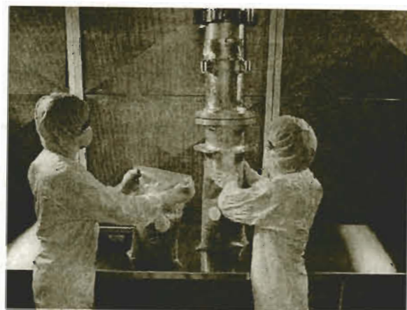
Figure 2. Bags filled aseptically with inoculated substrate. The filled bags then serve as individual fermentation vessels
