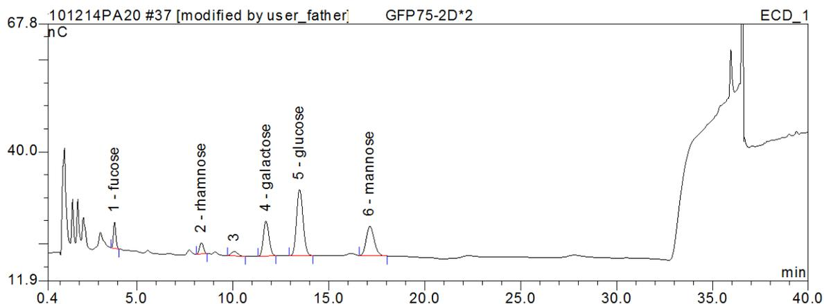
**Figure 6:** Ion chromatogram of the monosaccharide in GFP75-2D
