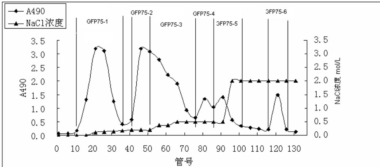
**Figure 1:** DEAE-Sepharose Fast Flow column chromatography of fraction GFP75
